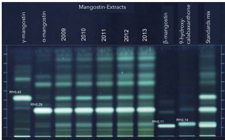
HPTLC RP-18 chromatogram at UV 366 nm after derivatization with NEU's reagent
